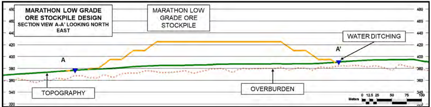
Figure DIET-08.2 Marathon Low-grade Ore Stockpile Design – Section View A-A' Looking Northeast
