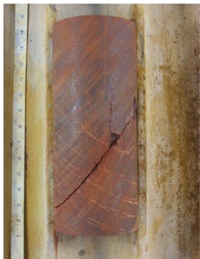
Figure 4: Rock sample RS-11 (iron oxide-massive) failed along a surface parallel to the banding structures
