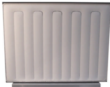
Laser-welded Flat Plate Membrane during Pressure Test
