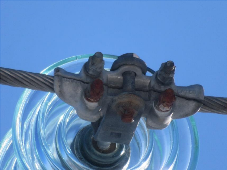
Figure 2 FleXall Clamp split from wear
