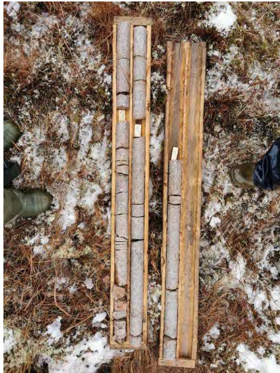
Photo 22: MW21-02 bedrock cores – 1.75 mbgs – 5.18 mbgs
