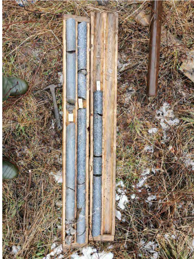
Photo 23: MW21-03 bedrock cores – 1.00 mbgs – 5.24 mbgs
