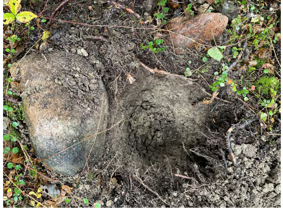
Photo 12 Overhead view of test pit (CKM-STP-003) showing dark grey gravelly clayey sand base.
