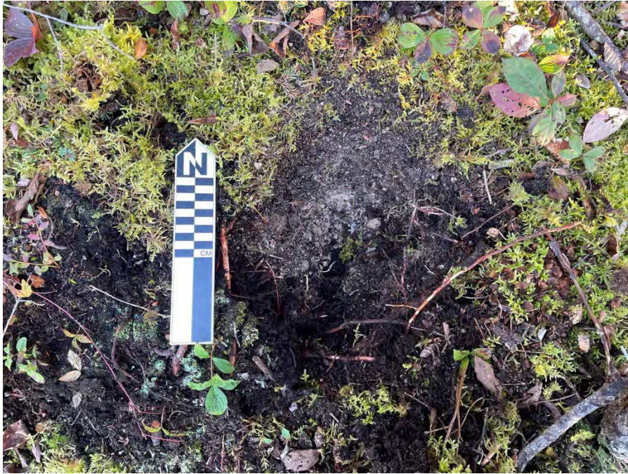
Photo 47 Overhead view of test pit (CKM-STP-007) showing gravelly clayey sand and unconsolidated shale bedrock base.
