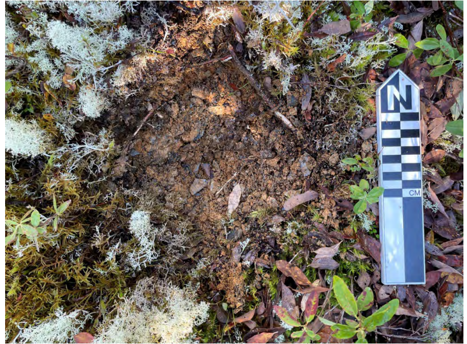
Photo 40 Overhead view of test pit (CKM-STP-006) showing light greyish brown gravelly sand and unconsolidated shale bedrock base.
