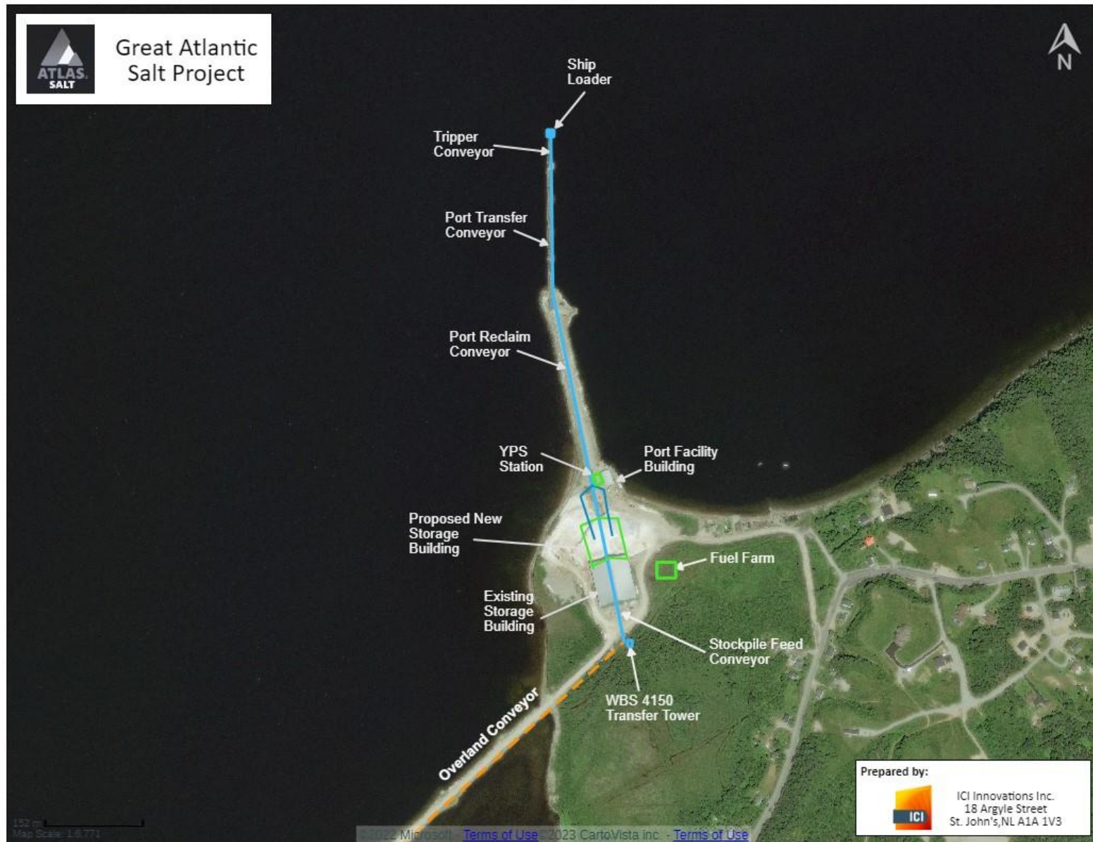
Figure 2.23: Turf Point Storage and Loading Modifications
