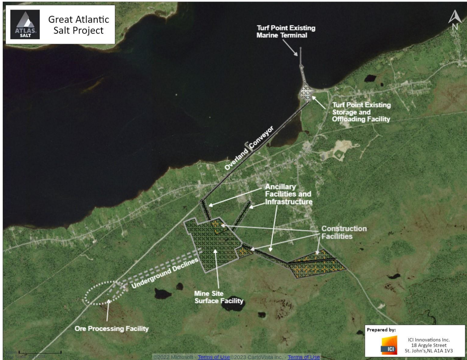
Figure 2.4: Overview of Key Project Components
