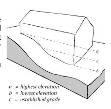
building, the average elevation of the finished grade of the ground immediately surrounding the structure, exclusive of any artificial embankment or entrenchment.
