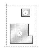
**LOT COVERAGE** means the combined area of all buildings on a lot measured at the level of the lowest floor above the established grade and expressed as a percentage of the total area of the lot.
