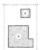
**LOT FRONTAGE** means the horizontal distance between side lot lines measured at the building line (the distance between points **A** and **B** in illustration at right).
