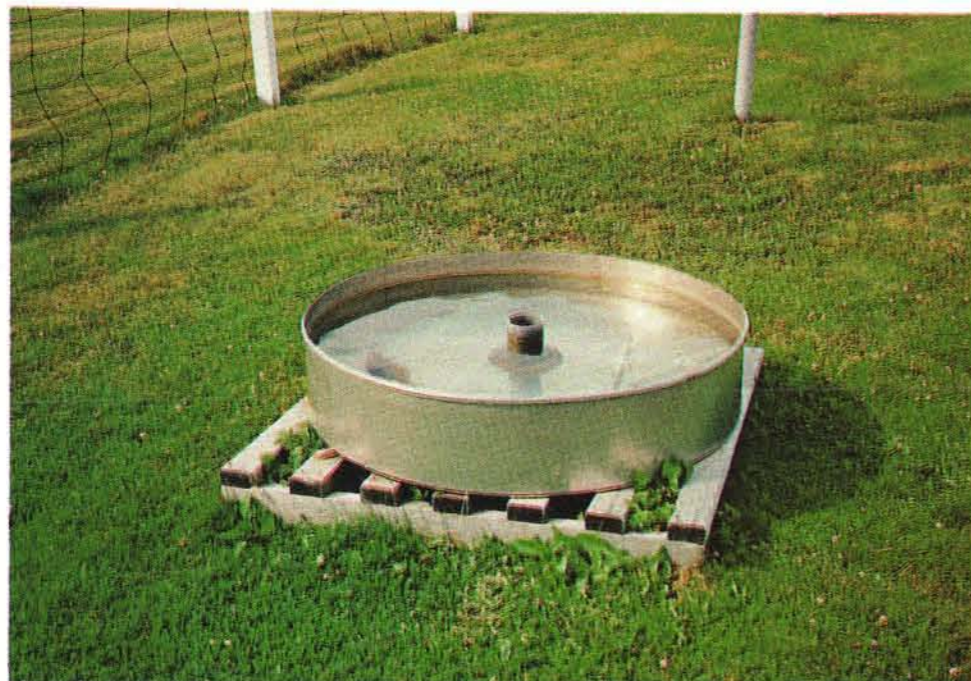
Figure 10.1 Class A Evaporation Pan
