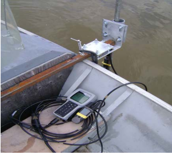
Figure 11: GPS Enabled Multi-parameter Probe Deployed from Side of Boat
