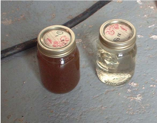
Figure 35: Water flushed from the St. Lunaire-Griquet distribution system during flushing (left), after flushing (right)
