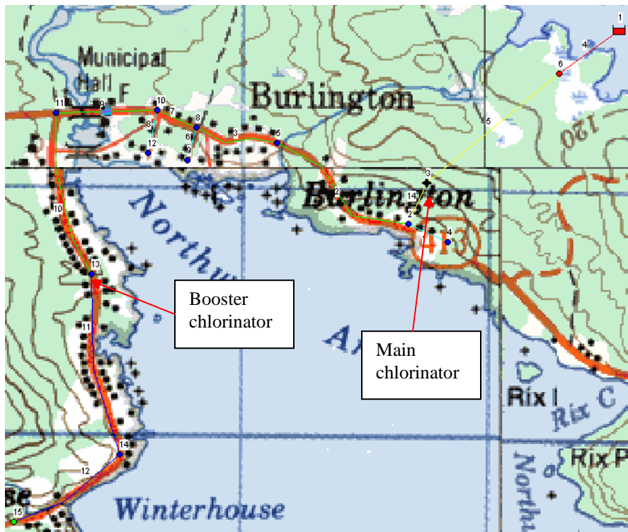
Figure 87: Optimal location of main and booster chlorinators in Burlington
