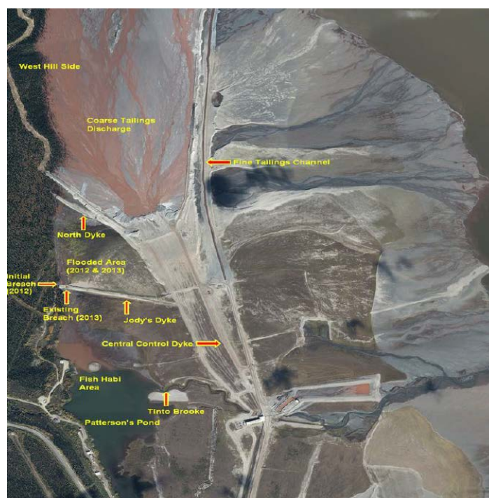
Figure 22: Jody's Dike – showing the location of the dike failure and the IOC Tailings System.
