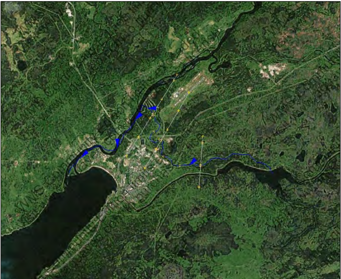
Figure 3: Screenshot from SMPDBK program showing flow-path (blue) and cross sections (light grey).
