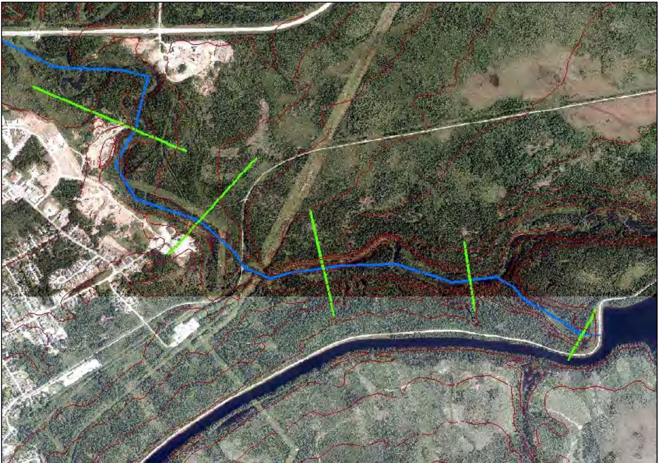
Figure 1: Cross sections (green) along initial portion of assumed flow path (blue) from Deep Bank Dam breach. Elevation contours shown in dark red.
