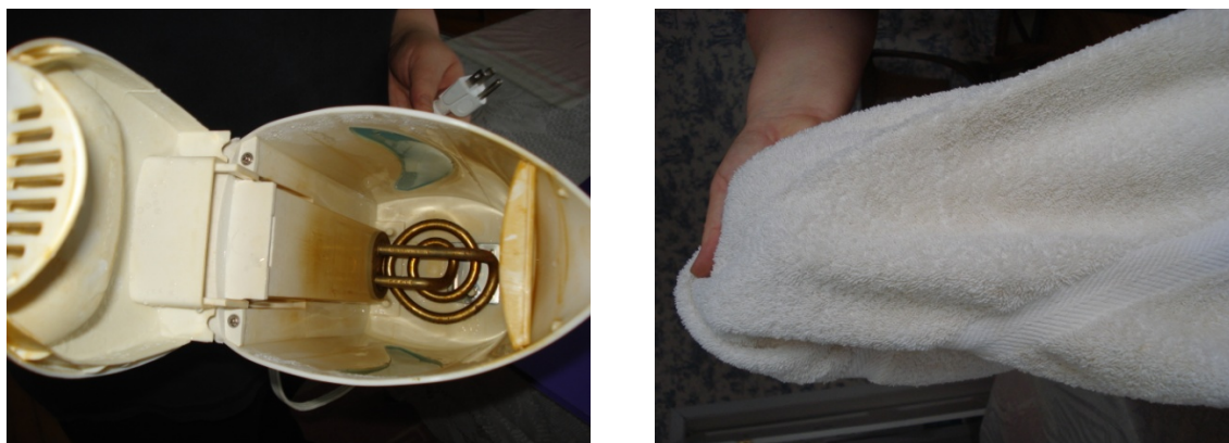
Figure 8.2 Iron Staining From Tap Water in Community F (Photos Taken in February 2010)
