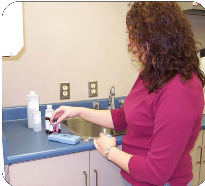
Watershed Management Specialist Deneen Spracklin measuring the chlorine residual of a THM sample.
