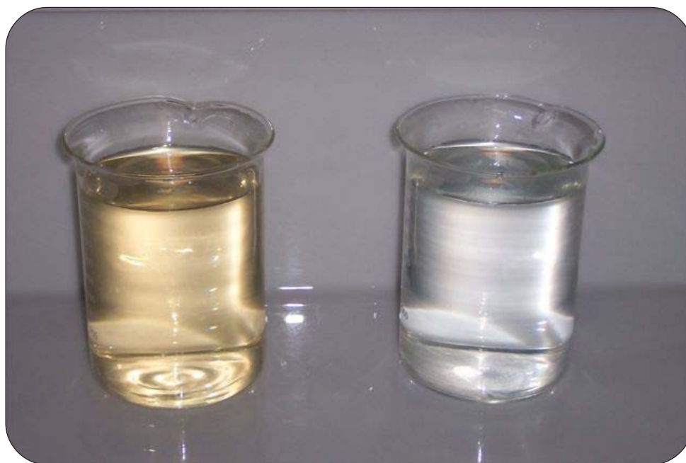
Raw water (left) and water after treatment (right) at the Clarenville water treatment plant. Photograph was supplied by Winston Lethbridge, Treatment Plant Operator.
