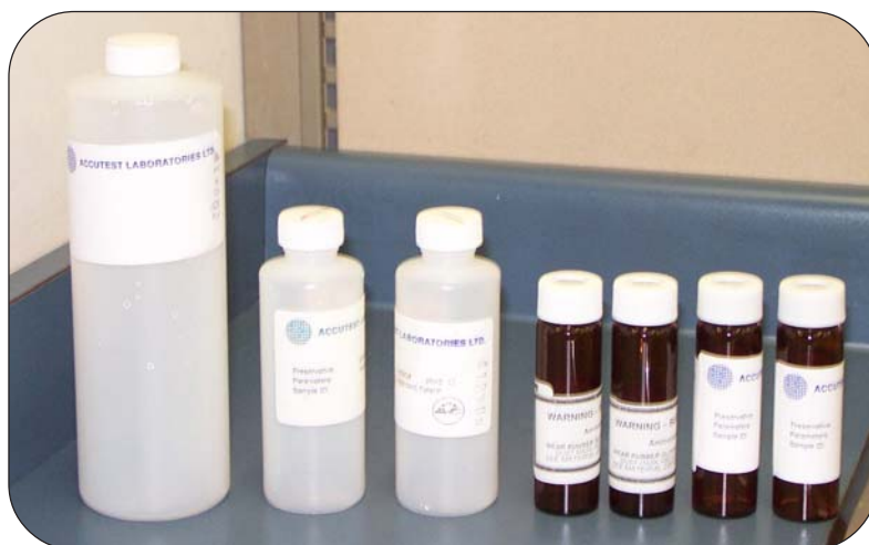
Bottles used for chemical and physical water quality sampling. From left to right, three plastic bottles for tapwater, two glass vials for HAAs and two glass vials for THMs.
