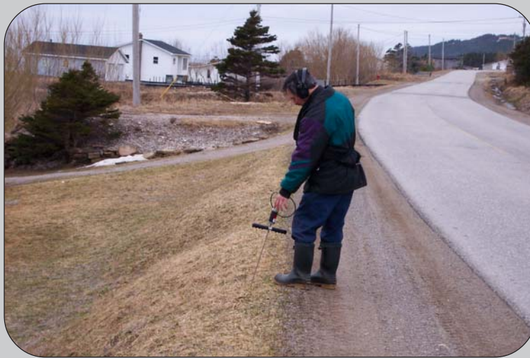
Operator Michael Snooks practicing leak detection during a leak detection training session in Cape St. George.
