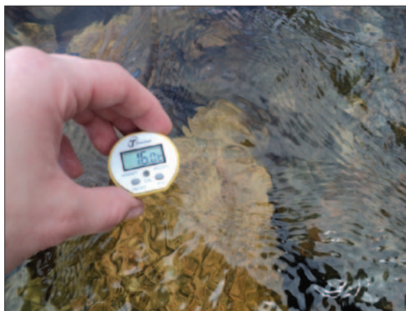
Taking a drinking water source temperature reading
