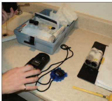
Preparing colorimeter to test for chlorine in tap water
