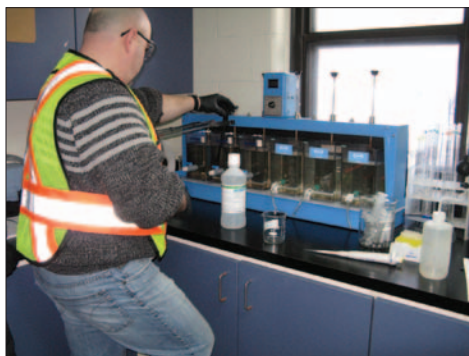
Operator performing a jar test to optimize coagulation-flocculation process
