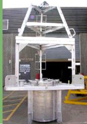
Aluminium superstructure and steel substructure.
