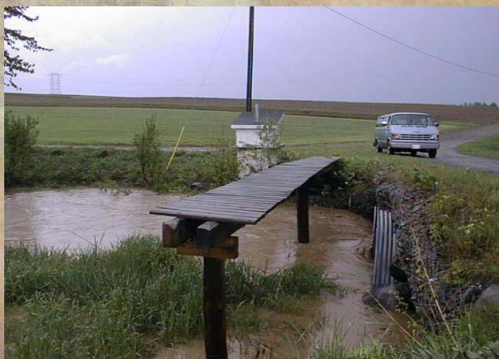
↙ Automated stage height recording and water sampling for flow, pH, conductivity, sediment loading, N, P, K, Ca, Mg →
