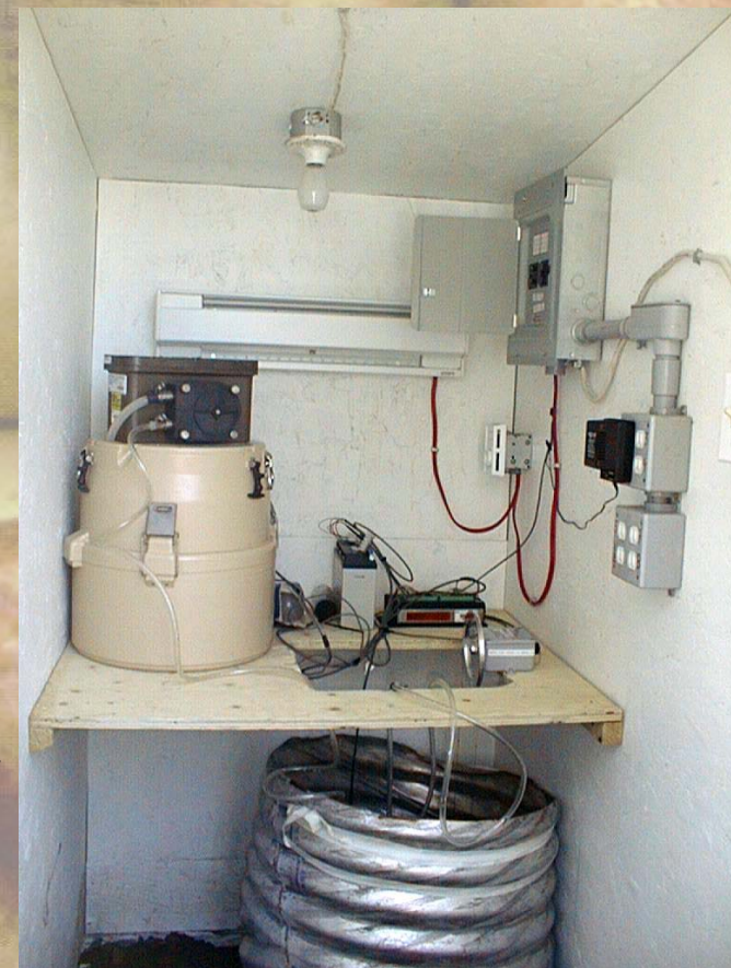
↙ Automated stage height recording and water sampling for flow, pH, conductivity, sediment loading, N, P, K, Ca, Mg →
