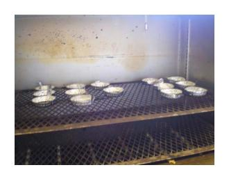
Filter (pore size = 1μm) is soaked in distilled water and dried at 103 °C.
