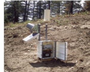
A. Precipitation gage (instrument detail) used in burned area at Missionary Ridge Complex Fire.
