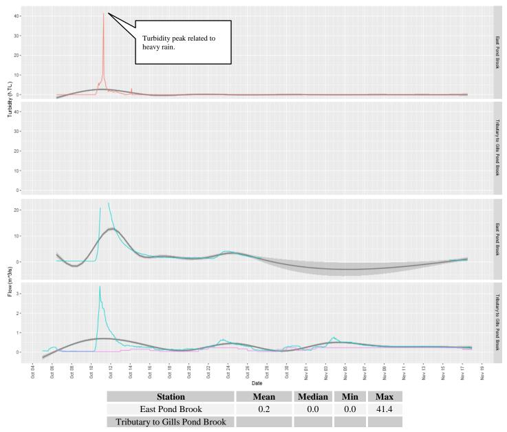
• Turbidity at EPB station was low for much of the deployment, except for a large increase following rain on October 10<sup>th</sup>. Turbidity quickly recovered in this case and exhibited a median value of 0.0 NTU for the duration.
