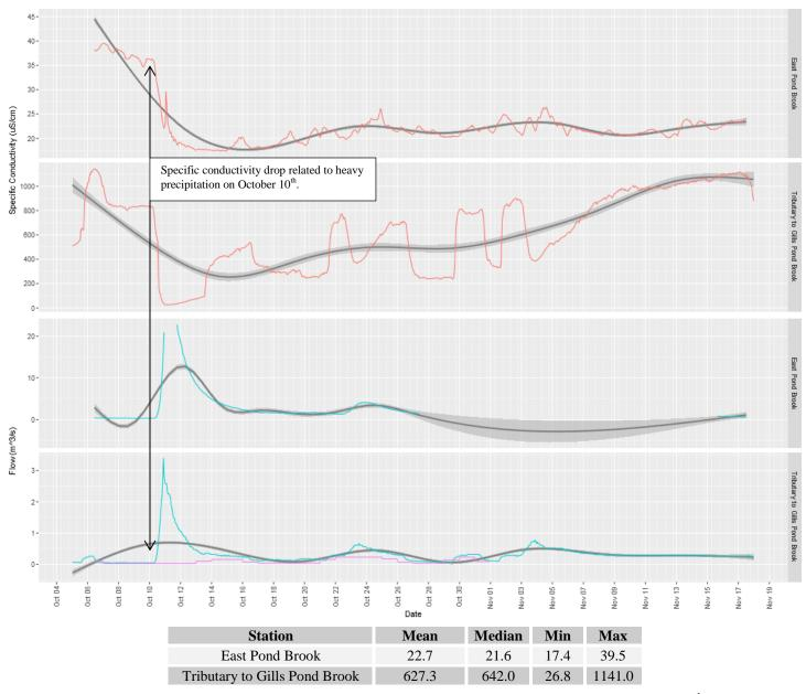
• Much like pH, specific conductivity was also driven down by heavy rainfall on October 10<sup>th</sup>. Recovery of pre-rainfall levels was relatively swift for TGPB due to the high level of dissolved solids in the effluent released into the stream. EPB station, however, was found to have a substantially lower specific conductivity at the end of the deployment than was observed at the start.
