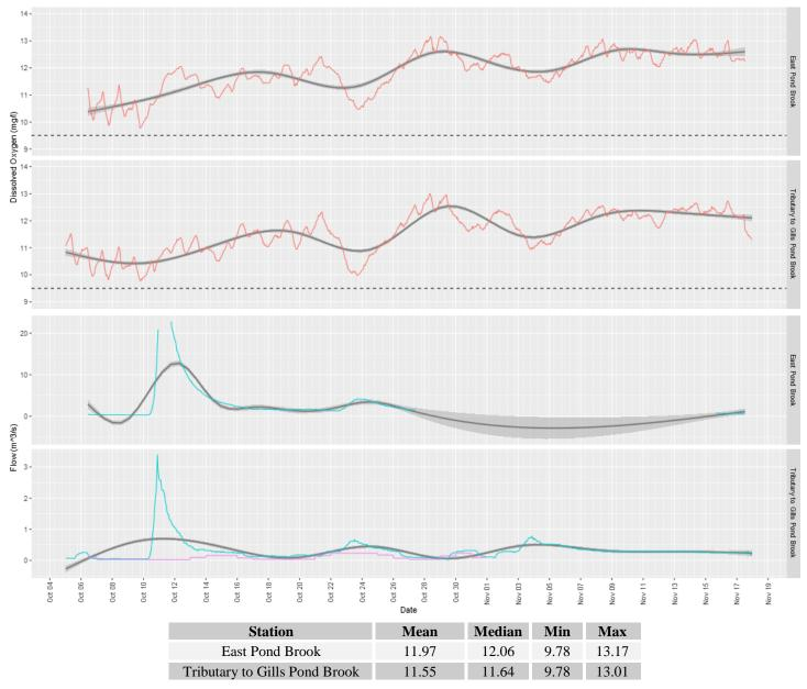
Dissolved oxygen levels increased throughout the deployment period as a result of cooling water temperatures. All values were found to be greater than the stated CCME guideline of 9.5 mg/l for the protection of cold water aquatic life.
