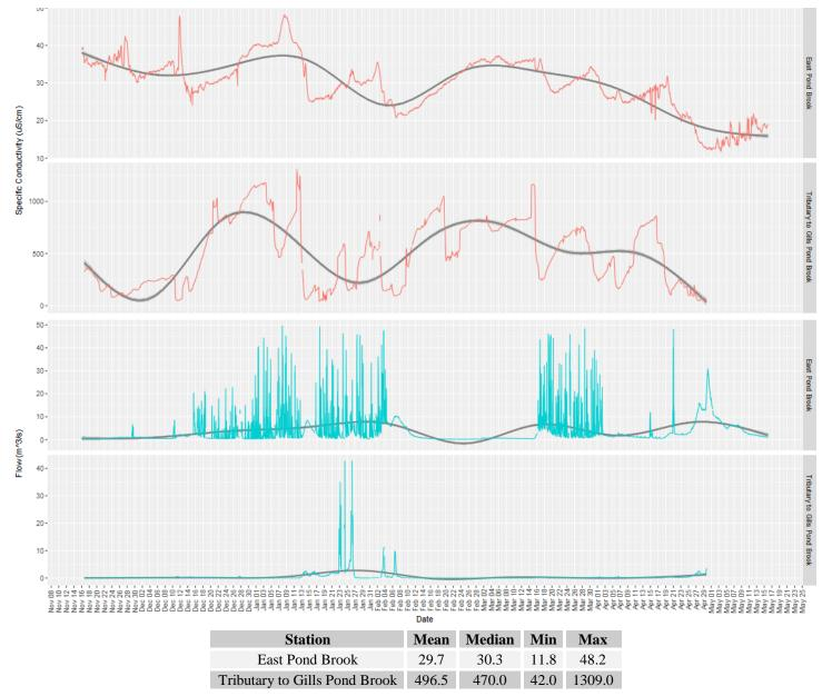
A downward trend in specific conductivity at East Pond Brook was observed while no substantial trend was seen at Tributary to Gills Pond Brook. In a 'pristine' environment such as East Pond Brook, the downward winter trend makes sense as dissolved solid inputs are minimalized due to frozen soils. Tributary to Gills Pond Brook, however, is largely fed by an effluent source where dissolved solids concentrations are controlled. A controlled effluence can be expected to remain relatively stable.
