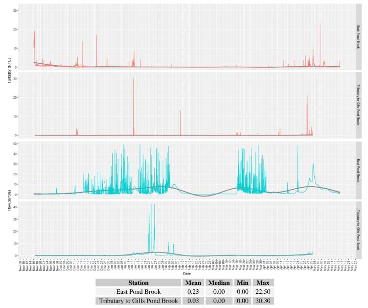
• Median turbidity levels at both monitoring stations were found to be 0.0 NTU during this deployment period, although a number of sporadic turbidity events were recorded over the course of nearly six months. No substantial turbidity events were encountered during the deployment interval.
