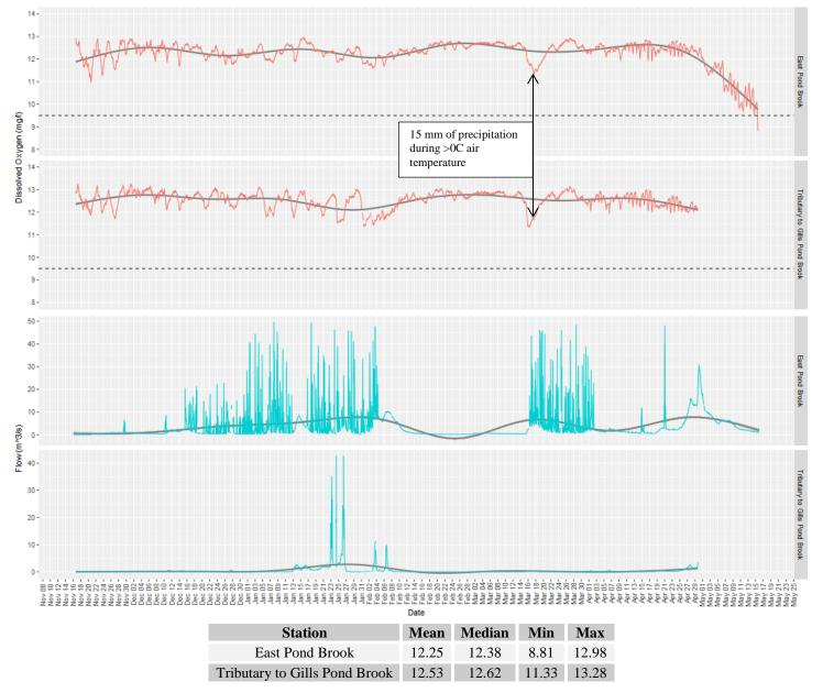
• Prior to the transmission failure at Tributary to Gills Pond Brook station, dissolved oxygen concentration trends appeared to be very similar between both stations. A sharp decline and recovery in DO concentration was seen in late during a weather event. A lag of nearly one day between DO low points both stations: Gills Pond Brook reached a minimum on March 18<sup>th</sup>, while East Pond Brook saw the minimum on March 19<sup>th</sup>.
