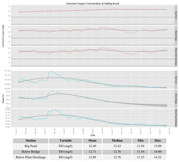
By December, dissolved oxygen saturation has generally approached its annual maximum – far above the CCME Guidelines for the protection of aquatic biota. Some fluctuations are present from time to time and are generally related to meltwater or influx of relatively warm precipitation.
