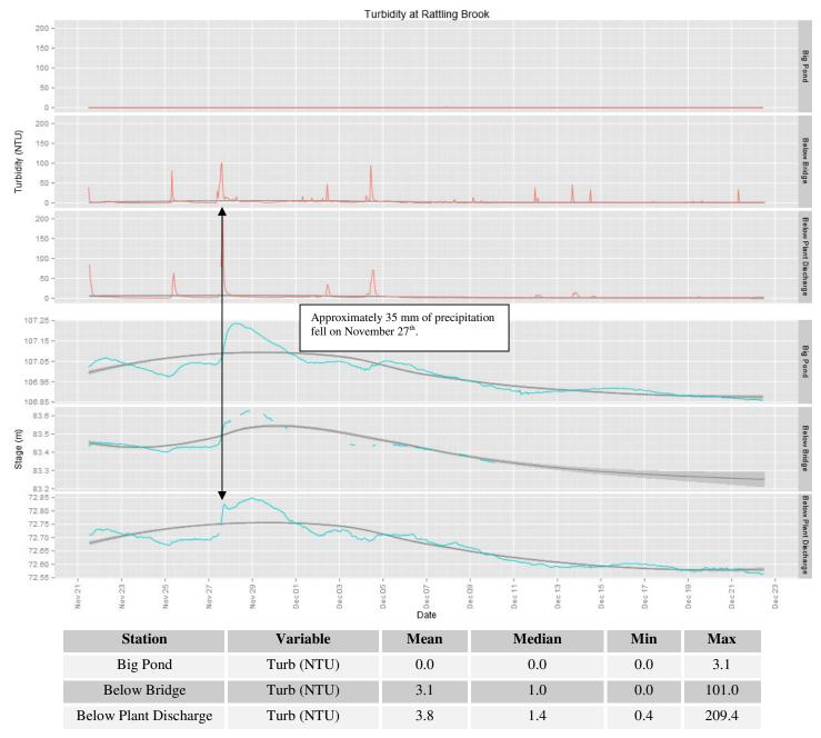
Eleven instances of turbidity greater than 40 NTU were observed at Bridge station during this deployment period while 14 were observed at Plant Discharge station. Two major turbidity events were observed at deployment on November 21<sup>st</sup> and another on November 27<sup>th</sup>, both during heavy rainfall periods.
