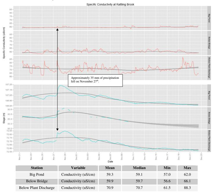
Specific Conductivity fluctuated at Bridge and Plant Stations, but showed no major trend upwards or down during the deployment period. Some peaks were identified and related to heavy precipitation.
