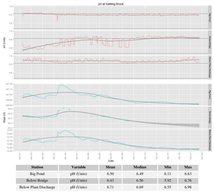
PH levels were mostly stable at Big Pond and Plant Discharge stations over the course of the deployment period while Bridge station showed a rise throughout the deployment. A series of rapid increases and decreases were observed at Bridge station as battery power came in and out. It appears that internal data from the Hydrolab used to fill gaps may be somewhat higher than data recorded by the datalogger. More investigation is needed.
