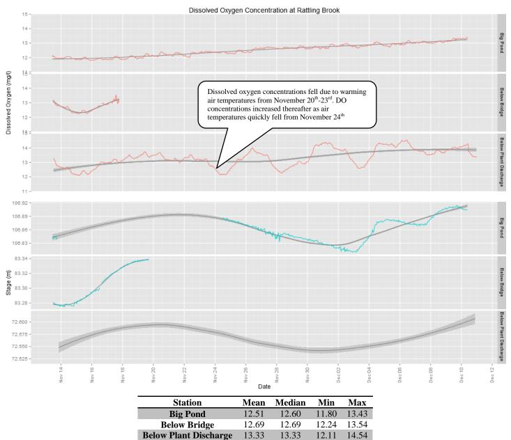
Dissolved oxygen concentrations increased slowly at Big Pond and Plant Discharge stations throughout the deployment period with some perturbations observed at Plant Discharge station
