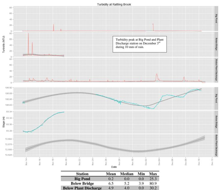
Turbidity levels were consistently low at Big Pond station throughout the deployment period. Plant
