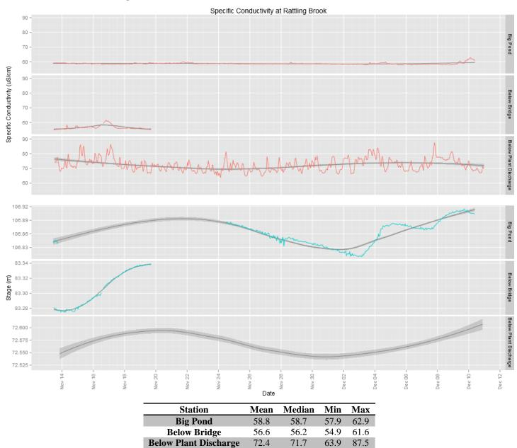
Specific conductivity was much higher and more variable at Plant Discharge station than upstream at Big Pond and Bridge station (for the little data available) because of discharge from settling ponds.
