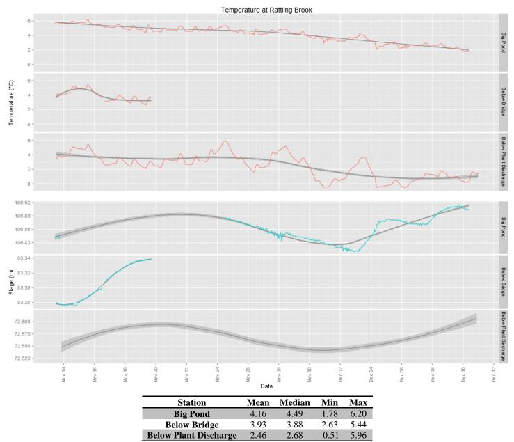
Water temperature fell continuously at Big Pond and Discharge stations throughout the deployment period as air temperatures decreased into late fall.
