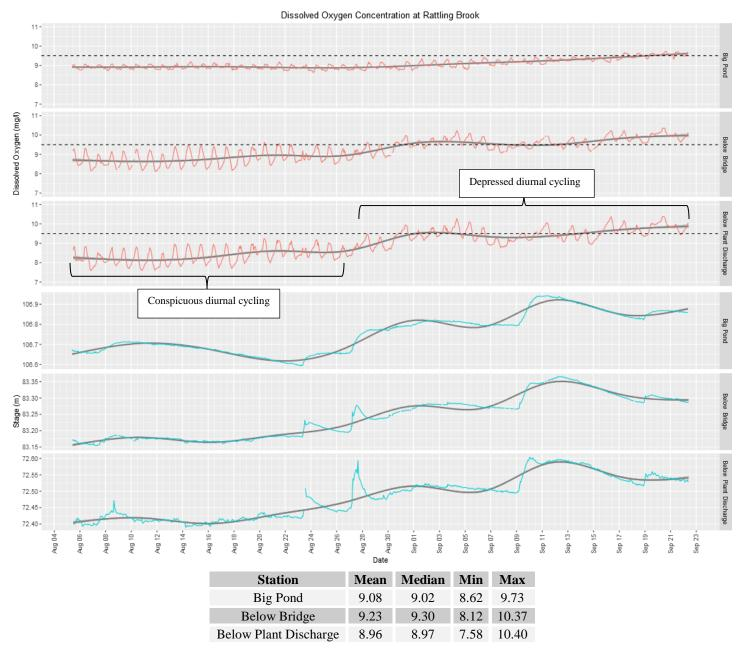
As water temperature declines, dissolved oxygen concentration increases. Early in the deployment period, diurnal cycling is conspicuous and drops in magnitude as the deployment period proceeds. This could be the result of aquatic productivity declining into the fall or as a result of rising water levels from precipitation.
