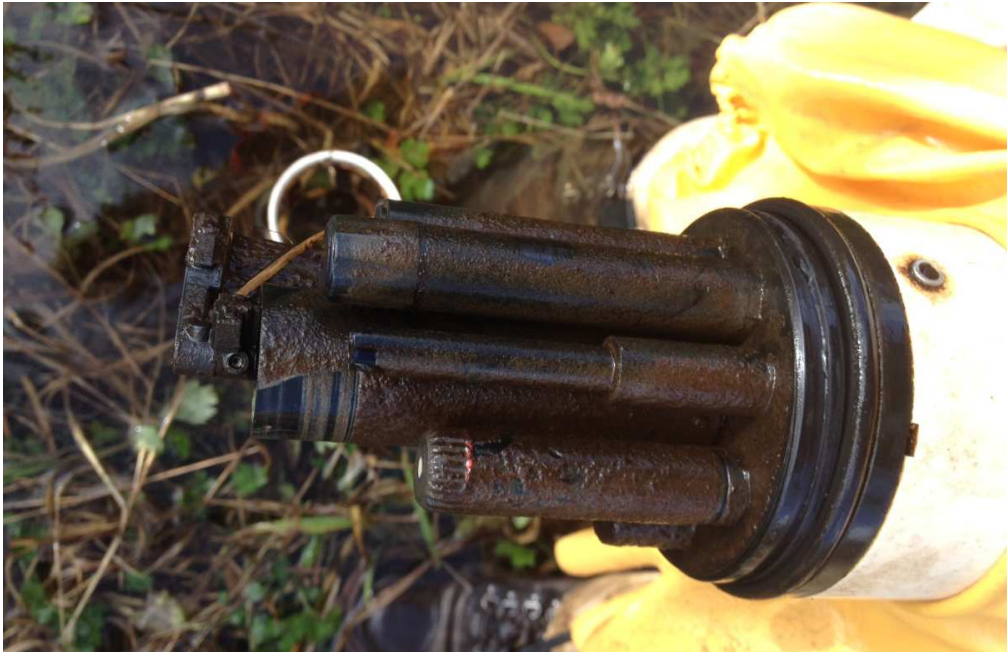
Figure A-9: Fouling on sensors after monthly deployment at Outer Cove brook at Clovelly Golf Course
