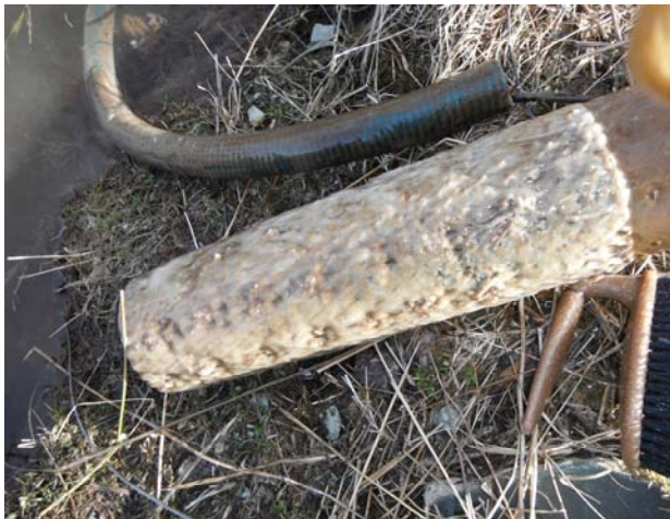
Figure 17: (a) Slime on sonde casing
