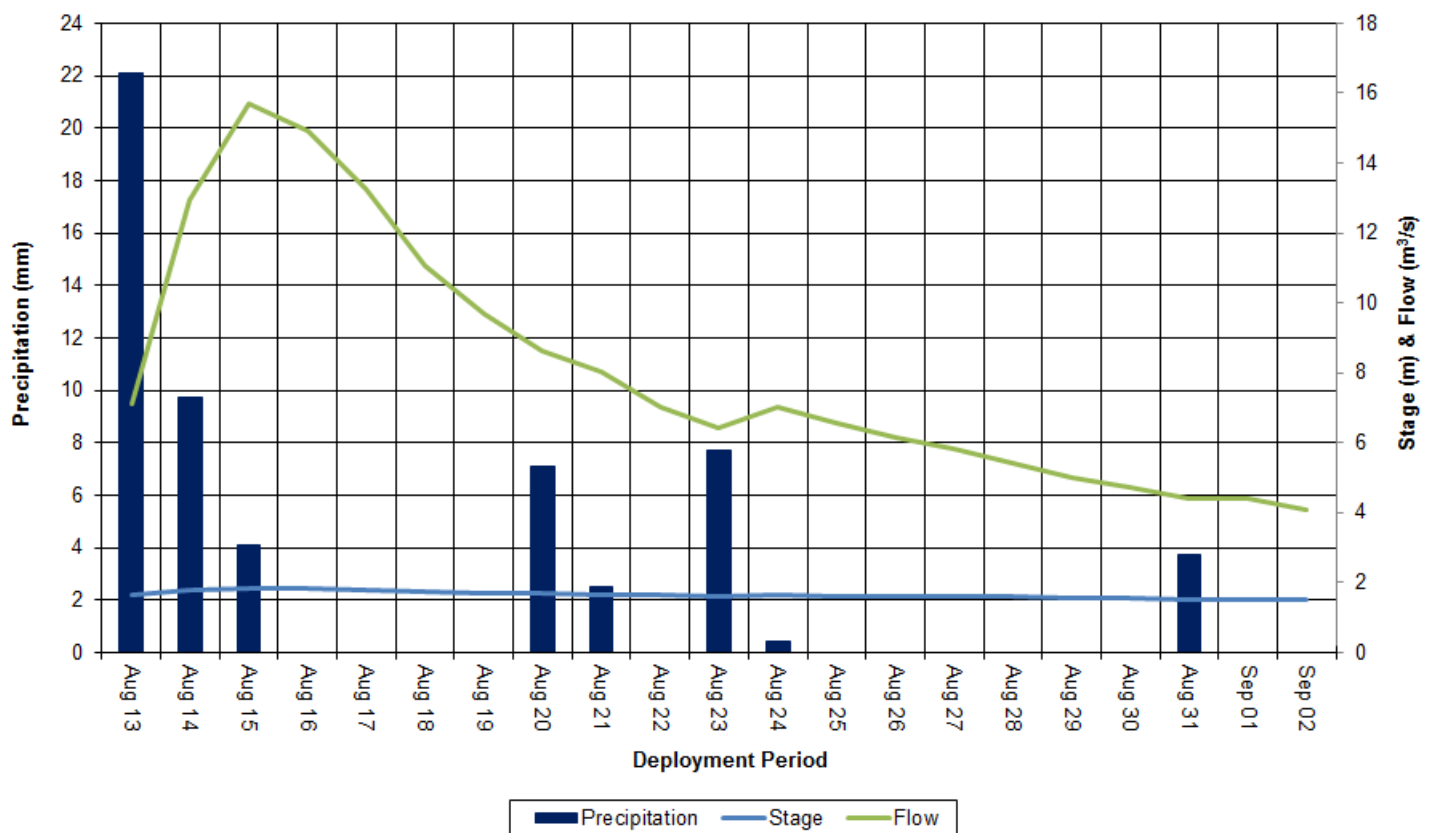
Figure 22: Daily Stage & Flow data from Reid Brook below Tributary and Total Daily Precipitation from Nain Weather Station
