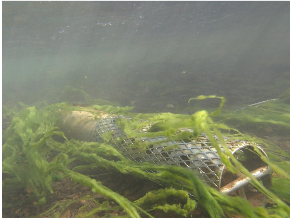
Figure 8. Algae were found attached to the instrument casing at the James Creek station on July 14, 2012. To prevent algae from affecting sensor readings, the instrument was covered by a thin nylon mesh (i.e., panty hose), before placing it in its protective metal casing.
