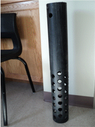
Protective casing for instrument
