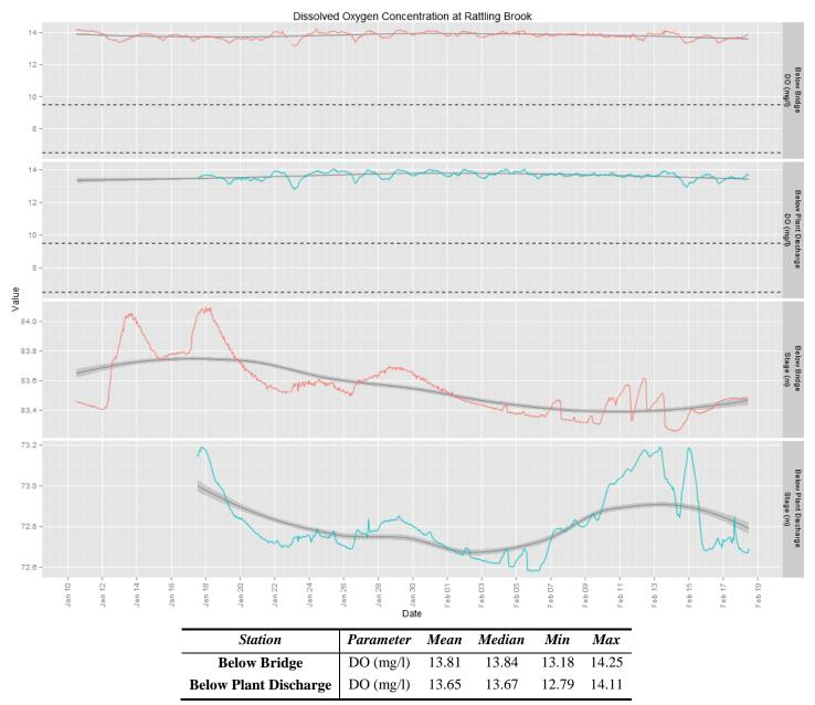
Dashed lines in the figures above indicate CCME Guidelines for the protection of early (9.5 mg/l O<sub>2</sub>) and other life stage (6.5 mg/l O<sub>2</sub>) cold-water biota. All dissolved oxygen levels were found to be above the CCME guidelines for the protection of early life stage aquatic biota (9.5 mg/l). Oxygen concentrations were
