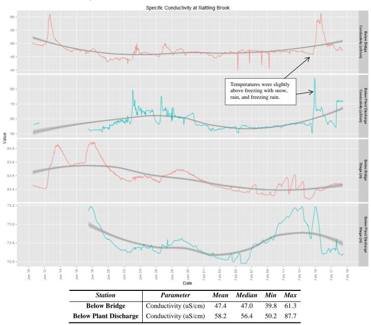
Conductivity peaked at both stations on February 14 - 15 during stormy conditions with snow and freezing rain. Precipitation inflow into the Rattling Brook river channel increases the concentration of dissolved solids.
