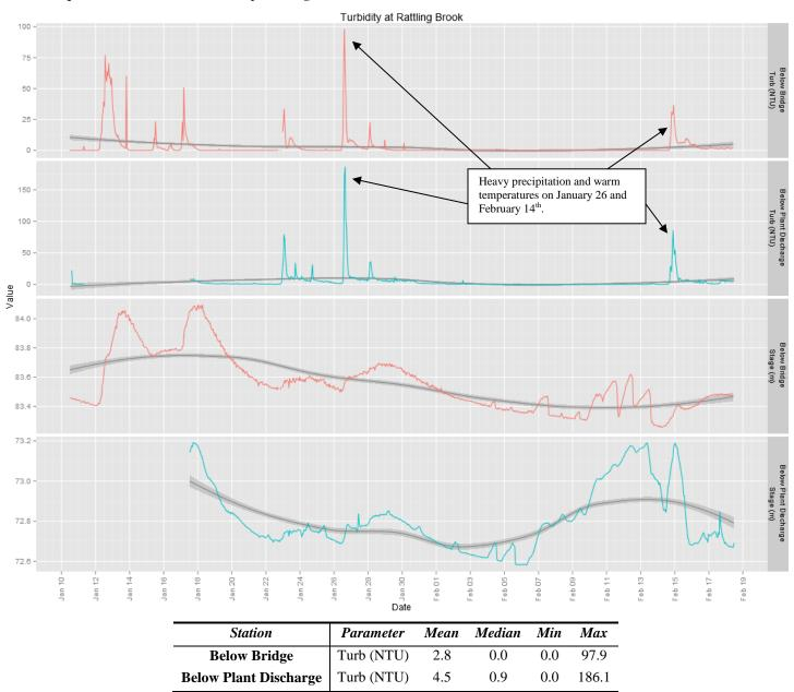
• The trend in turbidity is similar at both Bridge and Plant Discharge station, though the peaks are higher at Plant Discharge. Plant Discharge station intercepts the outflow from settling ponds draining the main plant site, which is a source of silt and sediment input into the Rattling Brook system.
