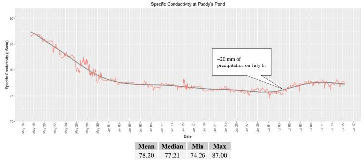
• Specific conductivity declined consistently through the deployment period indicating a decrease in dissolved solids at Paddy's Pond. A slight increase in the latter part of the deployment period appears to be a response to approximately 20 mm of rain on July 6.
