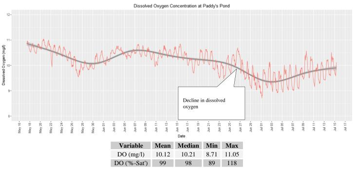
Dissolved oxygen concentration declined throughout the deployment period as water temperature increased. A notable perturbation occurred around June 27<sup>th</sup> when dissolved oxygen decreased. This decrease may be the result of a combination of warm waters (unusually warm daily temperature) and consumption by vegetative growth from an algae bloom.
