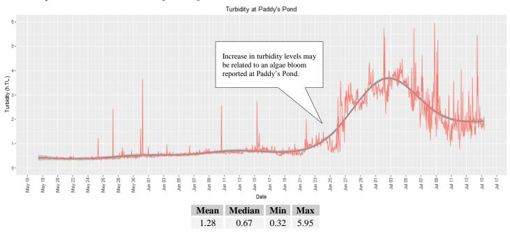
• Turbidity levels showed a small increasing trend with low variability from the beginning of the deployment to the end of June when there was a substantial increase. It was approximately at this time when reports were received about an algae bloom in the water body.
