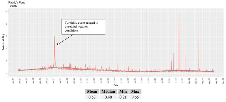
• Turbidity levels were low during this deployment period with and baseline turbidity levels were likely influenced predominantly by suspended algae and silt stirred up by wave action.
