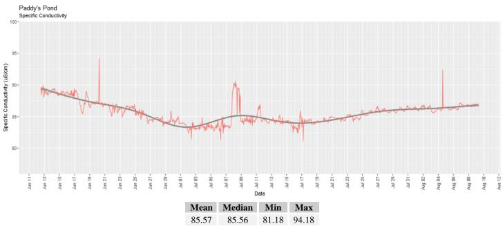
• For the first third of the deployment period, specific conductivity declined and reached a mid-deployment plateau. In the final third of the deployment conductivity slowly increased.
