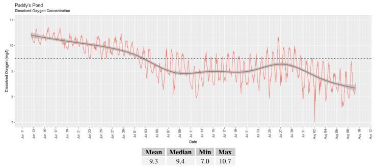
With increasing water temperature, dissolved oxygen concentrations declined over time. By July 2, DO concentrations were predominantly below the 9.5 mg/l guideline for the protection of early life stage cold water biota. This is expected for the time of year, as most aquatic organisms have developed beyond sensitive early stages by July.
