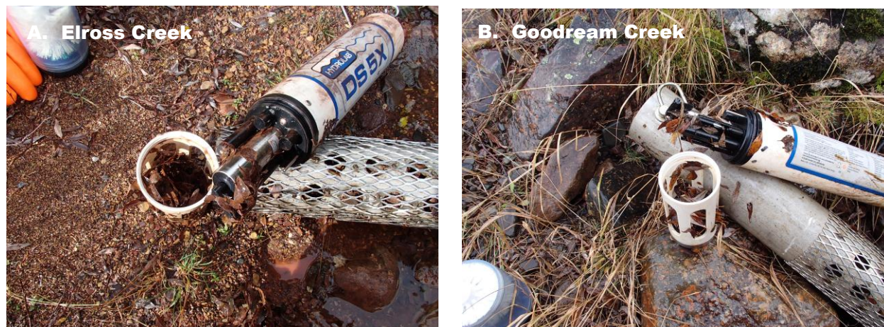
Figure 8. A mix of leaves and sediment were found tangled in and around the instrument sensors at (A) Elross Creek and (B) Goodream Creek on September 27, 2012.
