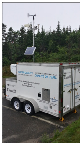
Figure 11: MEMP showing full mast setup
