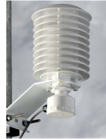
Figure 2: Temp/RH outfitted with Model 41003-X radiation shield
