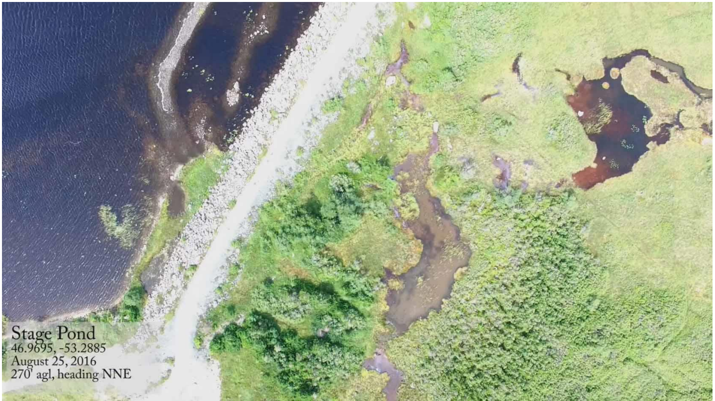
Photo 1: Potential seepage from the foot of Northwest Blackwoods Pond Spillway on Stage Pond
