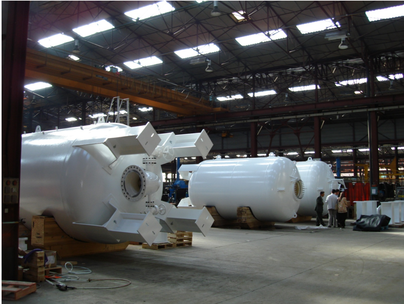
EUV 3x10,000 gallon 450psi Raw water inverted bladder surge vessels
