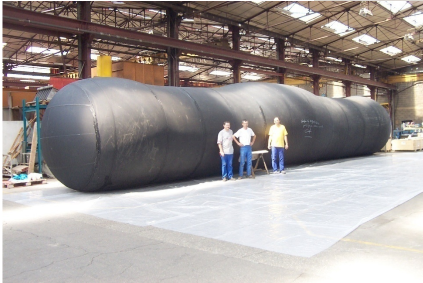
Hydrochoc 30,000 gallon potable bladder surge vessel Chicago
