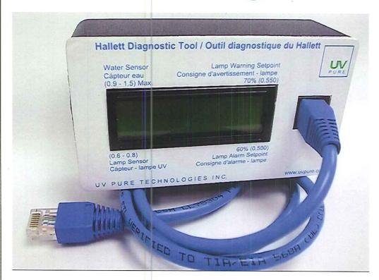
Simply plugs into right side of unit using an RJ45 Plug
