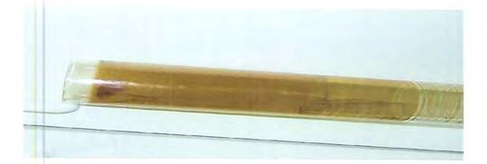
The presence of bacteria accelerates the rate of iron and hardness fouling (very common in wastewater/reuse)
