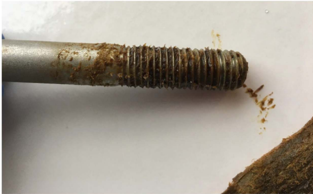
Figure 3: Stainless Steel bolt after a year of ASTM B117 Salt spray plus 6 months of ASTM G85 cyclic corrosion exposure
