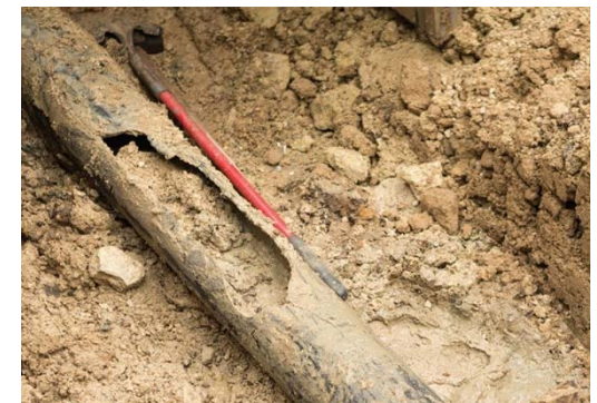
Pressure in lower end of system has been over 80 psi since fish plant shutdown
