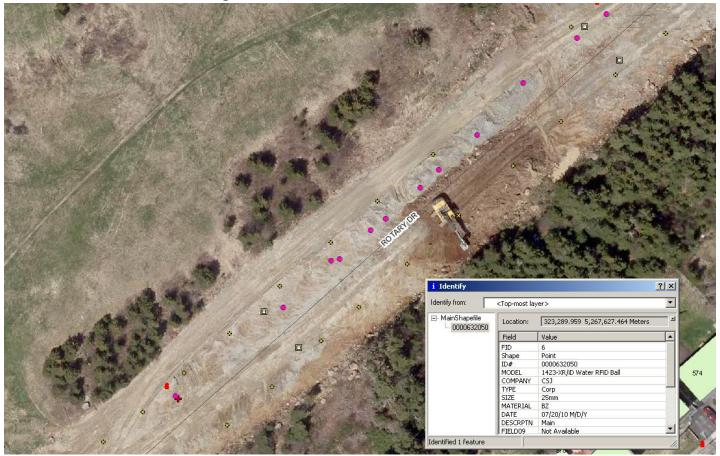
Data collected from Locator can be received by a GPS Unit and Transferred to GIS System
