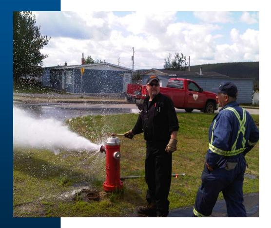
Flow testing along the 300 mm main line down hill from guy street
