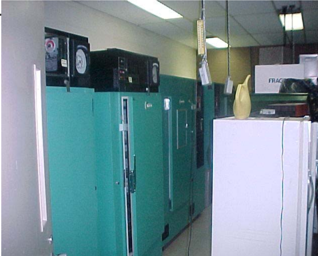
Growth Chambers using water for humidification
