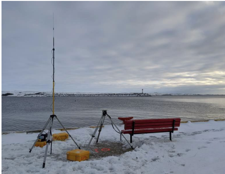
Figure 3.1.1 – Station de base GPS RTK Trimble installée sur le CSR1945 BS1f.
