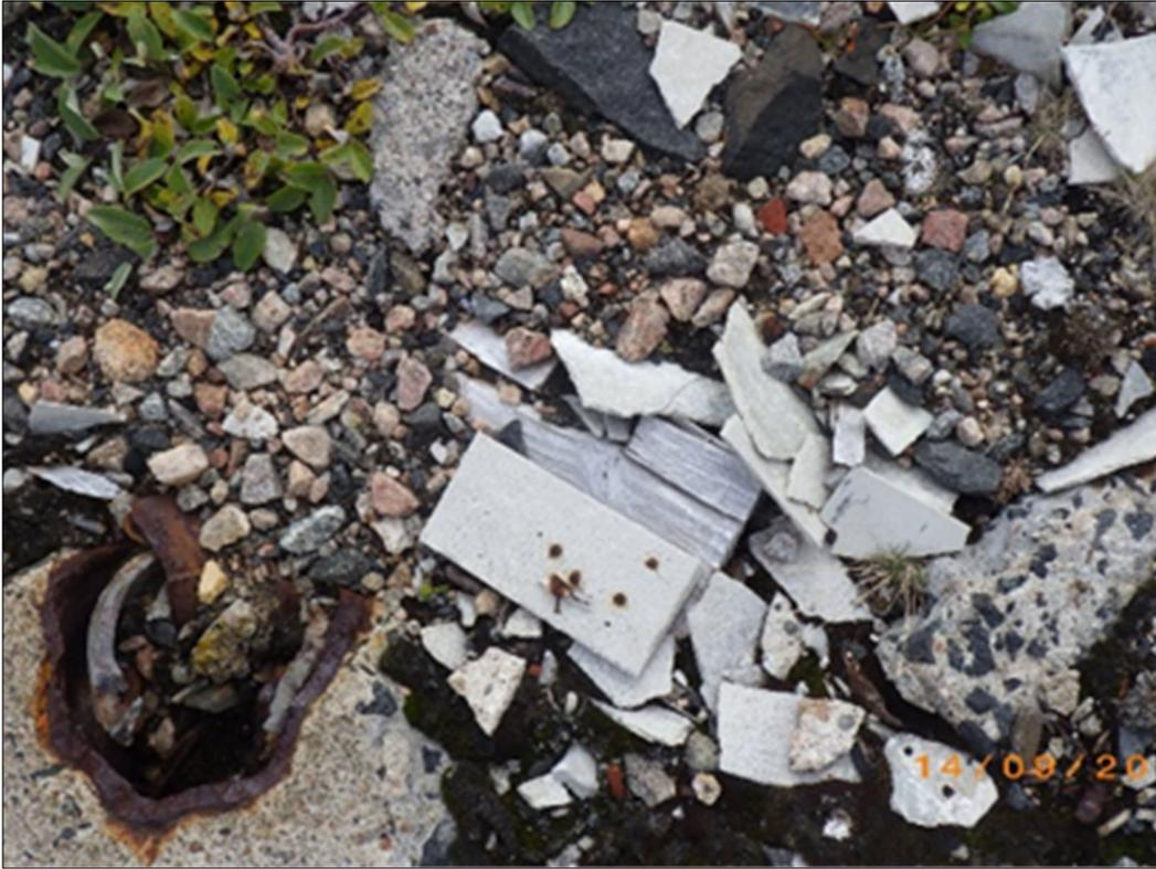
PHOTO 35 - APEC #5: View of potential ACM debris. (September, 2017)
