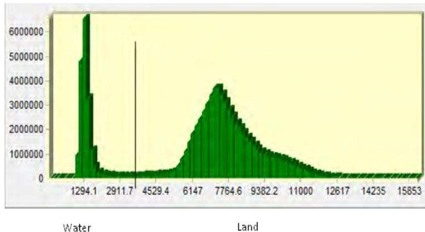
**Figure 5-2 Near Infrared Band Histogram – Water vs. Land Post-Processing / Accuracy Assessment (x-axis is the range of the available digital numbers and y-axis is the number of pixels in the image having a given digital number)**
