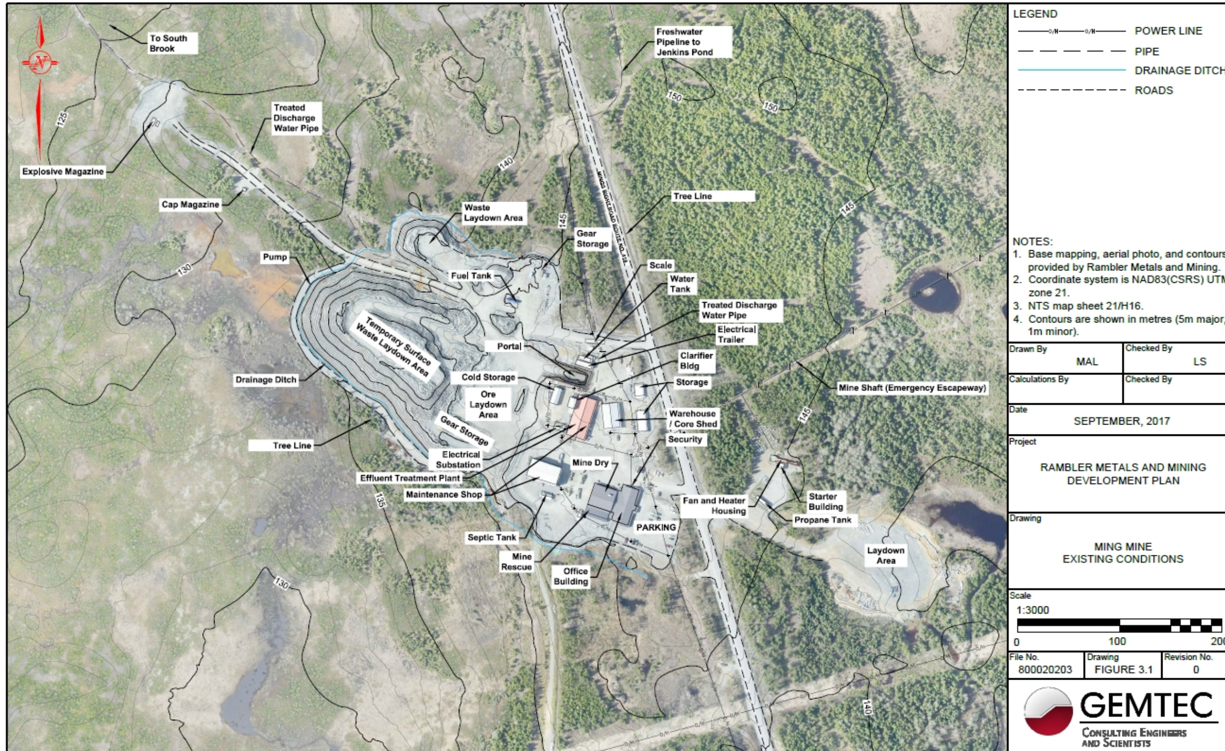
Figure 2-2 Existing Infrastructure at the Ming Mine Site
